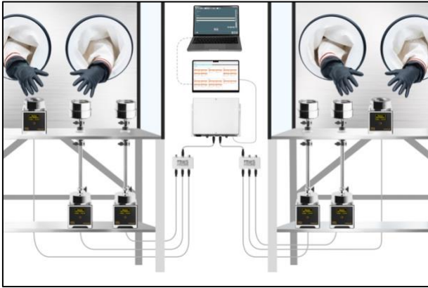
Example of GENIUS SYSTEM in 2 RABS isolators. The system is made by 2 GENIUS satellites and 4 GENIUS satellites with remote heads
