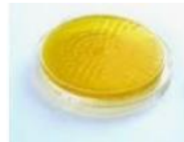
Figure 4) Impact holes on agar surface
